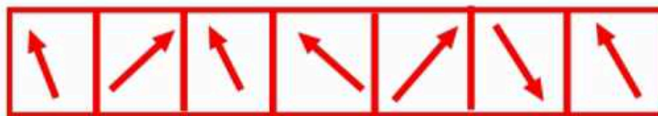
Dipole orientation in ferrielectric materials
