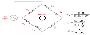
The Hay bridge differs from Maxwell's bridge by having a resistance R1 in series with a standard capacitor C1 instead of a parallel. The term W appears in the expression for both Lx and Rx. which indicates that the bridge is frequency sensitive.
