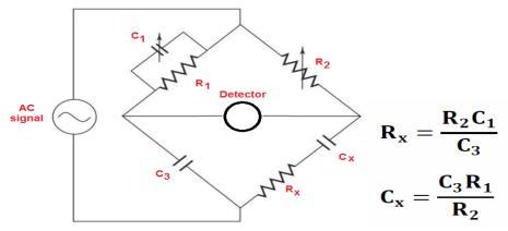
Used for the measurement of capacitors.
