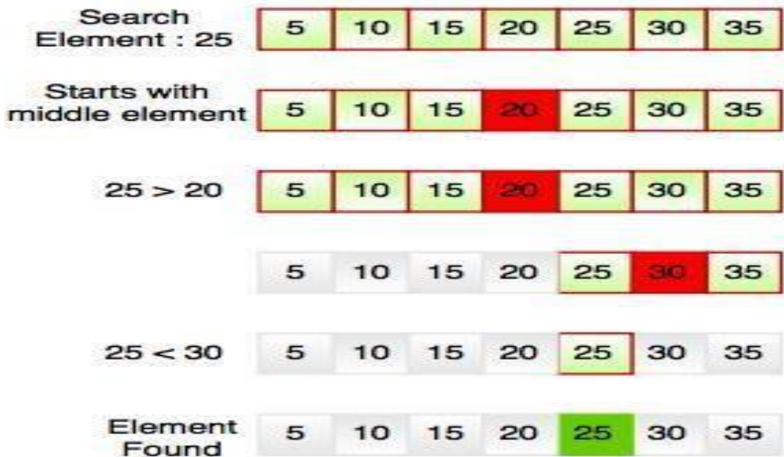
Fig. Working Structure of Binary Search
