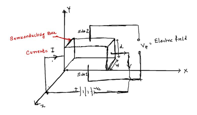
Consider the figure shown above. Here Current I is in the positive X-direction. Magnetic field B is in positive Z-direction then induced electric field will be in the Negative y-direction.
