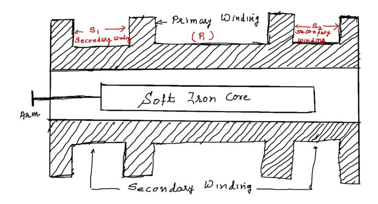
The transformer consist of a single primary winding P1 and Two Secondary windings S1 and S2, which is wound on a hollow cylindrical former.
