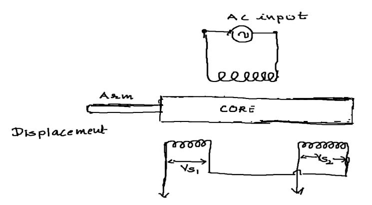
The movable soft iron core slides within the hollow former and therefore it affects the magnetic coupling between the primary and the two secondaries. The displacement to be measured is applied to an arm attached to the soft iron core. Actually the core is made up of a nickeliron alloy which is slotted longitudinally to reduce eddy current losses. When the core is at normal position I .e at null position then EQUAL voltages are induced in the two secondary windings.
