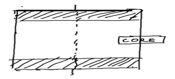
In figure (b), the core is at 0, which is central zero or null position. Therefore  $Vs_1=Vs_2$  and Vo/p=0
