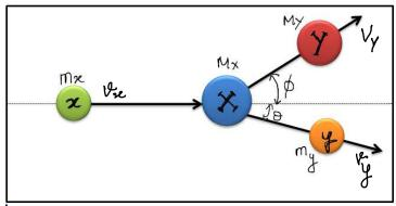
From D My Vy sin  $\phi$  = My Vy cos  $\phi$  -  $\Theta$ From D My Vy sin  $\phi$  = my Vy sin  $\phi$  -  $\Theta$ Squaring D and  $\Theta$  and adding them we get  $(m_{x}v_{x})^{2}+(m_{y}v_{y})^{2}-2m_{x}v_{x}m_{y}v_{y}\cos \phi=(m_{y}v_{y})^{2}-G$
