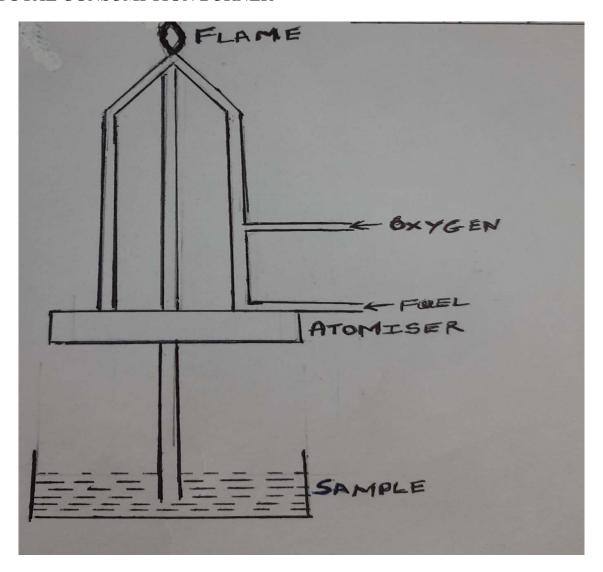
The fuel gas burns in presence of oxygen to produce a flame.
