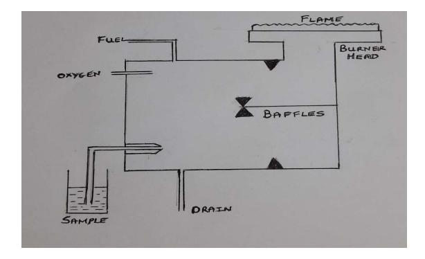
The fuel,oxidant and the liquid sample are thoroughly mixed before entering the flame hence its known as pre – mix burner. Only the small droplets reach the flame. The large droplets are trapped by baffles and drained off. Hence 5% of the sample is introduced in the flame which produces efficient atomisation but emission intensity is weak. The flame produced is stable, non – turbulent, noiseless and large in cross-section.
