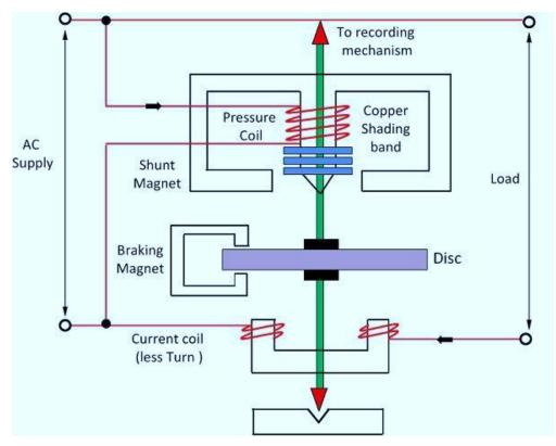
• The flux produced by this magnet is proportional to, and in phase with the load current.
