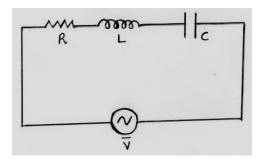
In general impedance  $\overline{Z}$  is always greater then R in series LCR circuit and hence the peak value of current  $I_{omax}$  is always less than  $\frac{E_O}{R}$
