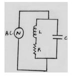
When admittance is minimum, the impedance will be maximum and the current in the circuit will be minimum.
