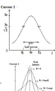
side of resonant frequency  $f_0$  where current falls to  $i_0/\sqrt{2}$ .
