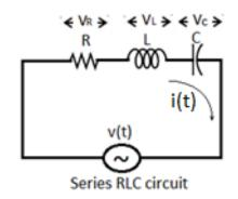
current by  $90^{\circ}$  and voltage across capacitor lags current by  $-90^{\circ}$
