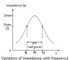
For ideal components Q- factor is equal to voltage amplification factor
